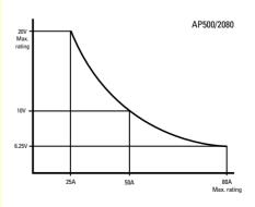
These compact autoranging bench or systems power supplies use a switch-mode topology to provide a wide range of adjustable voltage and current combinations within a 1 kilowatt power envelope.
