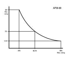
These compact autoranging bench or systems power supplies use a switch-mode topology to provide a wide range of adjustable voltage and current combinations within a 3 kilowatt power envelope.
